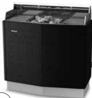
SDK 10 Intended to be combined with separate control panel type TS 16, TS 30 or CC and relay box RB 30. 10.7 kW output. A steam distributor for Tylarium can be added to SDK/SD. Item no. 6430 1009
